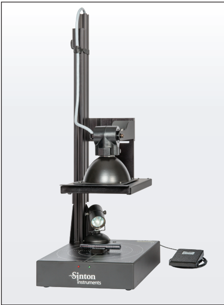
The Mini Boule Tester allows for quick characterization of the true bulk lifetime of miniature silicon boules using the transient PCD measurement method.
